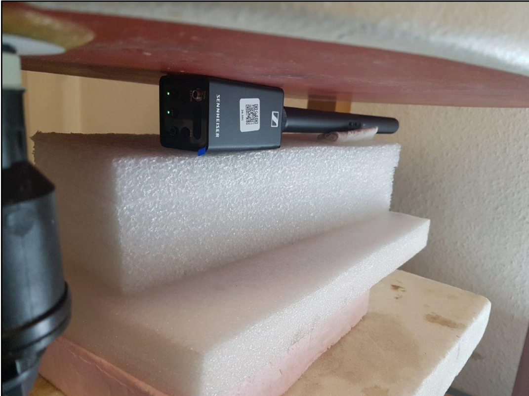
Photo 7: Test position - Left side with 0mm distance
