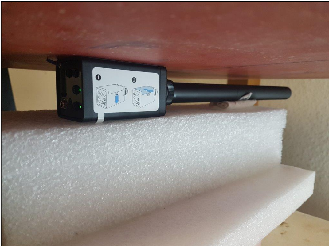
Photo 8: Test position - Right side with 0mm distance
