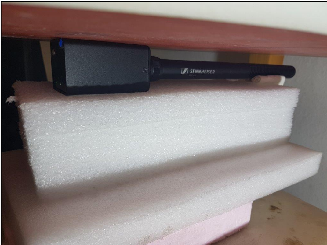
Photo 6: Test position - Front side with 0mm distance
