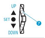
In the selection mode of the "TUNE" menu, press the multi-function switch ⑦ (switch position ●SET). The current channel number appears on the display and then the currently assigned frequency is displayed.
