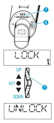
To achieve this, either press the ON/OFF button 8 or the multi-function switch 7 (switch position •SET).
