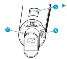
Briefly press the ON/OFF button (3). The LED ON/LOW BATT (10) lights up and the standard display is shown on the display panel (6); after a short pause, "RF" appears on the display panel (6). The LC display remains backlit for approx. 20 seconds.
