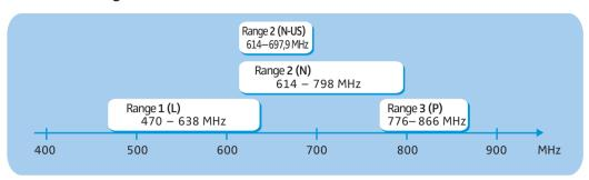
The transmitter has two frequency banks:
