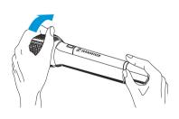
Unscrew the microphone head by turning it in the direction of the arrow.
