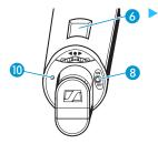
To switch the radio microphone on, briefly press the red button 8.
