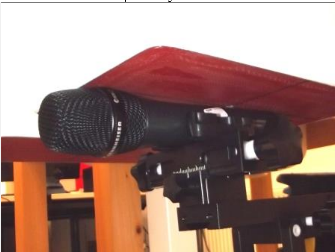
Photo 14: Test position – right side with 0mm distance
