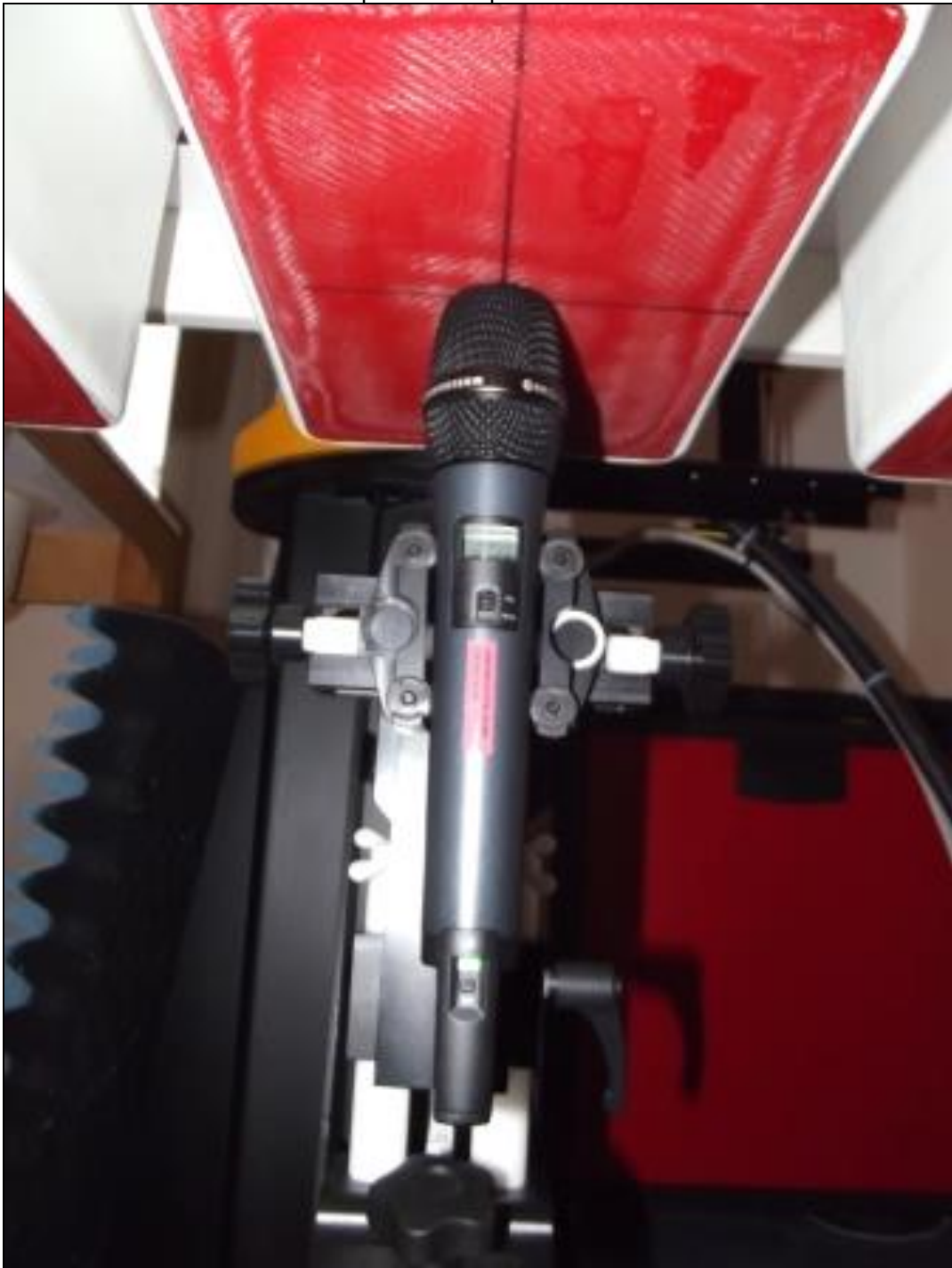
Photo 15: Test position – top side with 0mm distance
