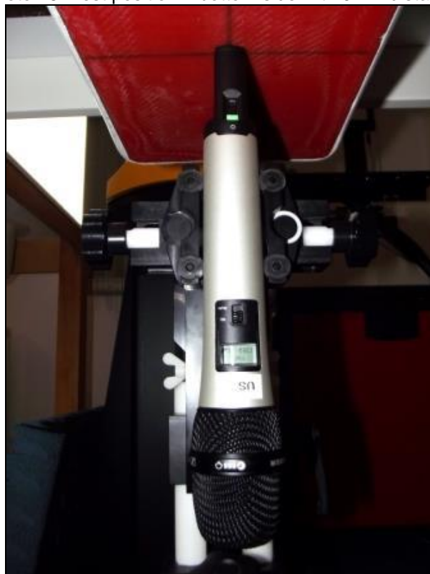
Photo 16: Test position – bottom side with 0mm distance
