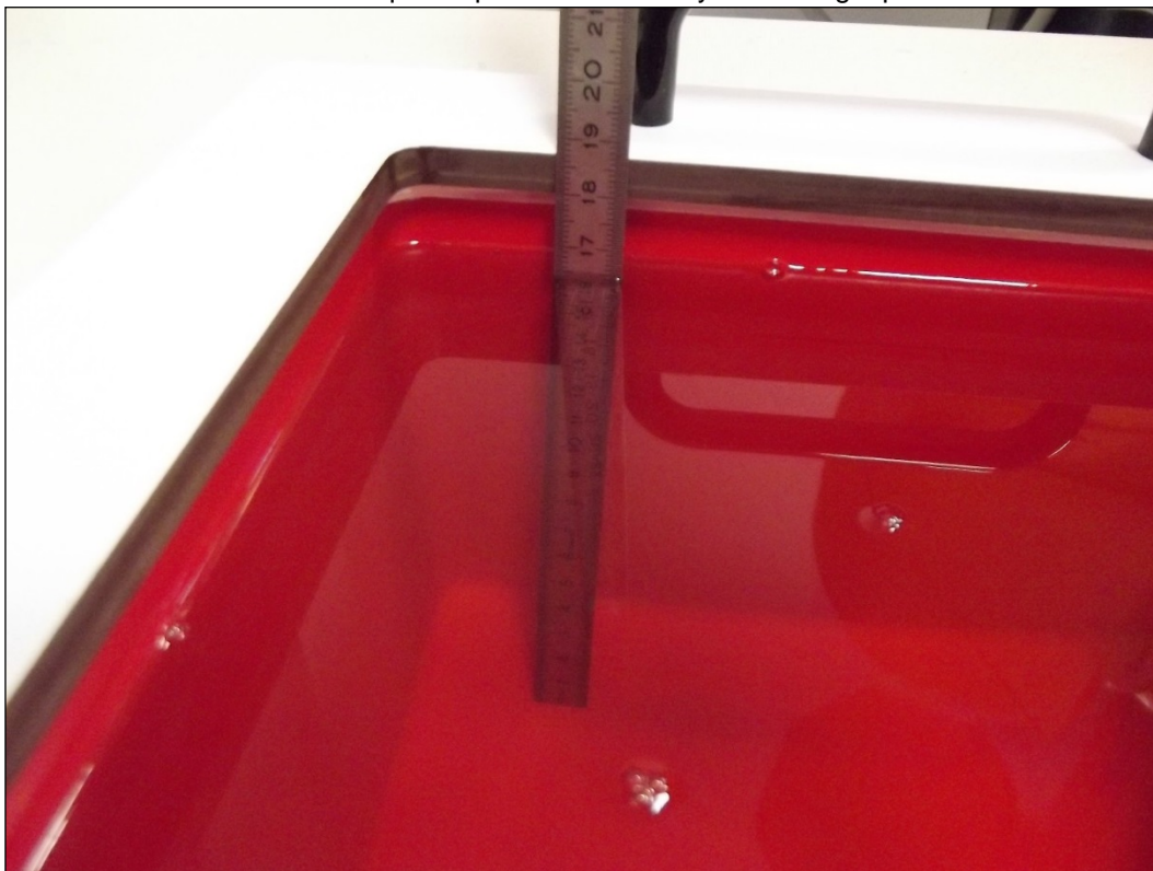
Photo 1: Liquid depth 450 MHz body simulating liquid
