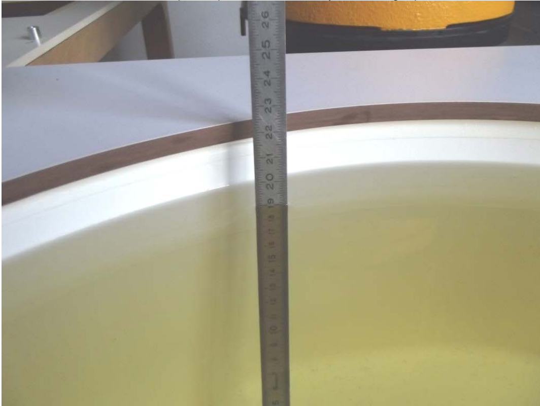
Photo 1: Liquid depth 2450 MHz body simulating liquid
