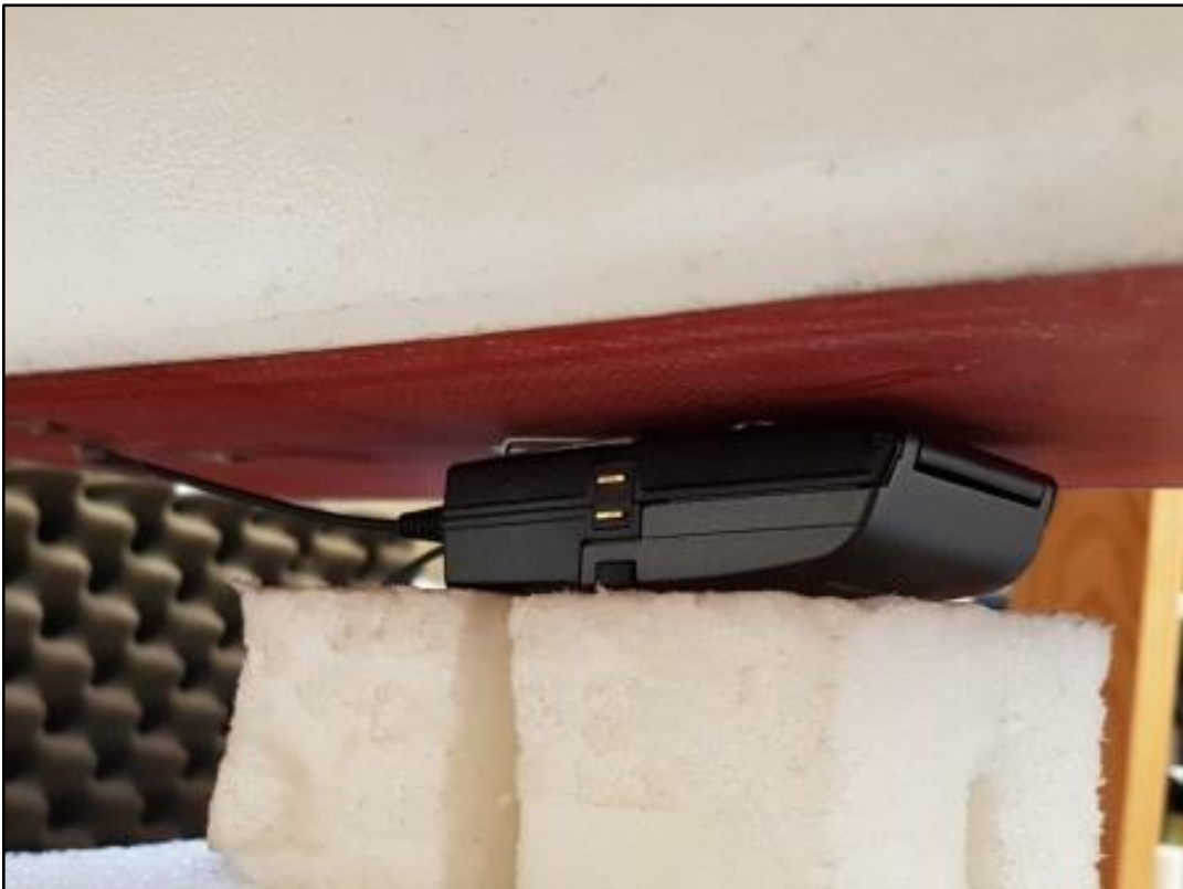
Photo 8: Test Position - Rear with 0mm distance
