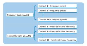
Each of the channels in the frequency banks "1" to "20" has been factorypreset to a fixed transmission frequency (frequency preset). The factorypreset frequencies within one frequency bank are intermodulation-free. These frequencies cannot be changed.
