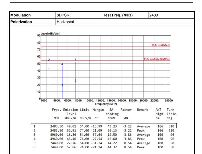
Note 2: Margin (dB) = Emission level (dBuV/m) – Limit (dBuV/m).
