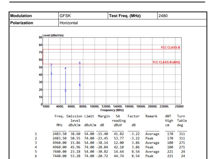
Note 2: Margin (dB) = Emission level (dBuV/m) – Limit (dBuV/m).
