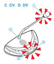
When the chairman assigns you the "speaking right", your microphone switches on. The microphone LED @ and the signal light ring @ light up red. The loudspeaker @ is muted. Depending on the conference mode and the speaker limit set, the microphone of the previous speaker will be switched off.
