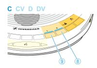
The loudspeaker volume is changed. As long as you keep the key @ or @ pressed, the LED next to the key lights up.
