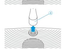
Carefully pull the gooseneck microphone out of the microphone socket 4.
