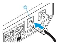
► Connect the DC power supply ⊚ to the socket ᡚ.
