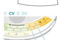
▶ Press the selection key A ⑧ or the selection key B ⑨ to trigger circuits via a home controller.
