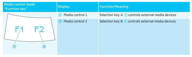
The display has an automatic brightness control. Approx. 4 seconds after the last key press, the brightness will be reduced. With each key press, the display will light up with maximum brightness.
