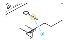
The charge status indicator 36 goes of after approx. 5 seconds. The LED 3 then display the status of the charging electronics.
