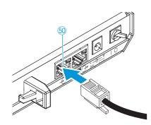
Connect the system cable to one of the six RJ 45 sockets ("PORT 1-6") of the SDC 8200 CU-M or SDC 8200 CU central unit (see page 70 and the instruction manual of the SDC 8200 conference and interpretation system).
