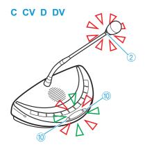
The initialization process starts. All conference units that are operational show a microphone LED (10) flashing green and red and a signal light ring (2) flashing red.
