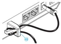
Pass the cable of the DC power supply through the cable grip 49 as shown.
