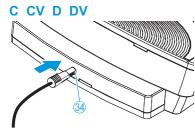
Slide the battery pack into the battery guide rails 33 of the conference unit.
