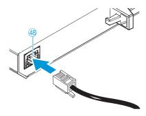
Connect the supplied network cable (Cat5) to the network socket (RJ 45) 48.
