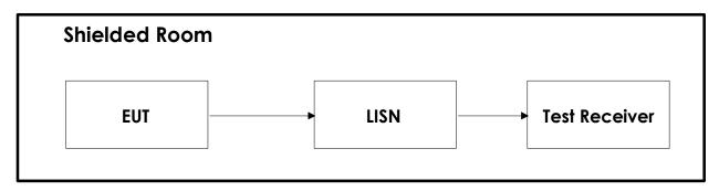
Test Set-Up 5
