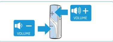
If you have set a very high volume level and switch the receiver off and on again, the volume is reset to a moderate level to protect your hearing.
