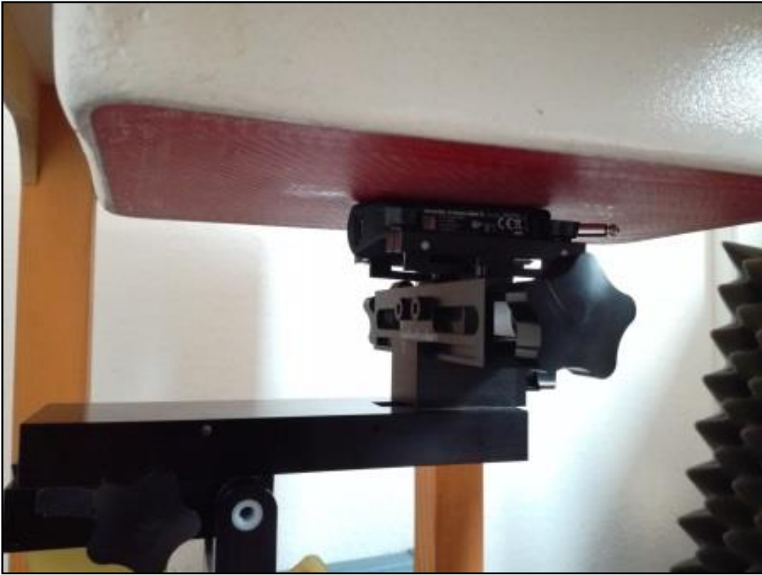
Photo 8: Test position - TX 63 - Bottom with 0mm distance
