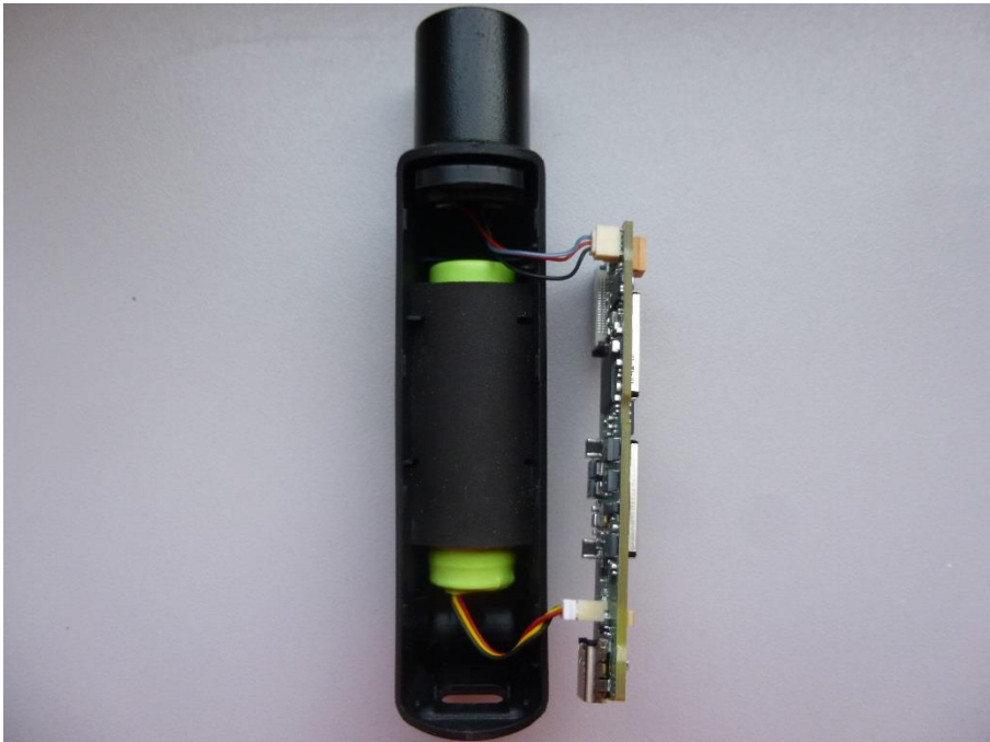
Photo 10: RDs front cover removed
