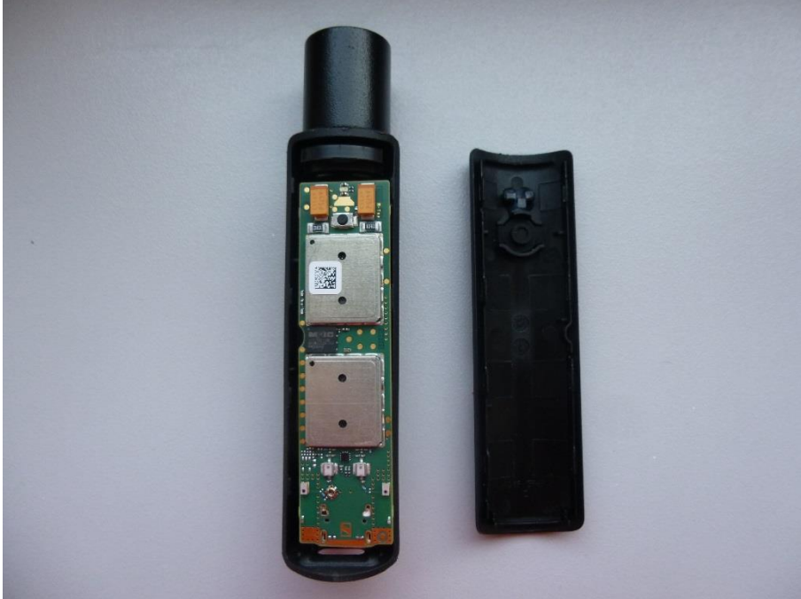
Photo 9: RDs front cover removed
