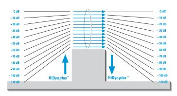
This transmitter is equipped with HiDyn *plus* the Sennheiser noise reduction system that reduces RF interference. It increases the signal-to-noise radio in wireless audio transmission to more than 114 dB.
