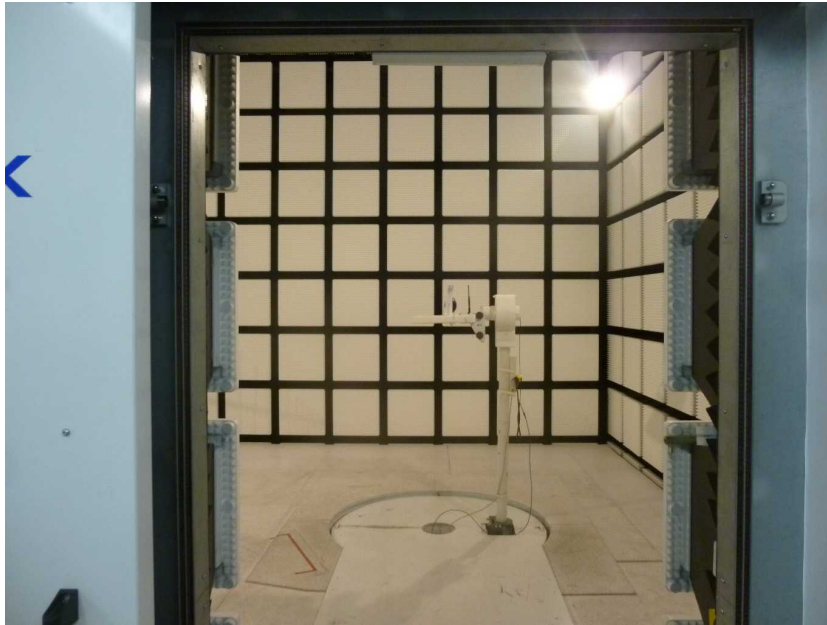
Photo 1: EUT at the anechoic chamber
