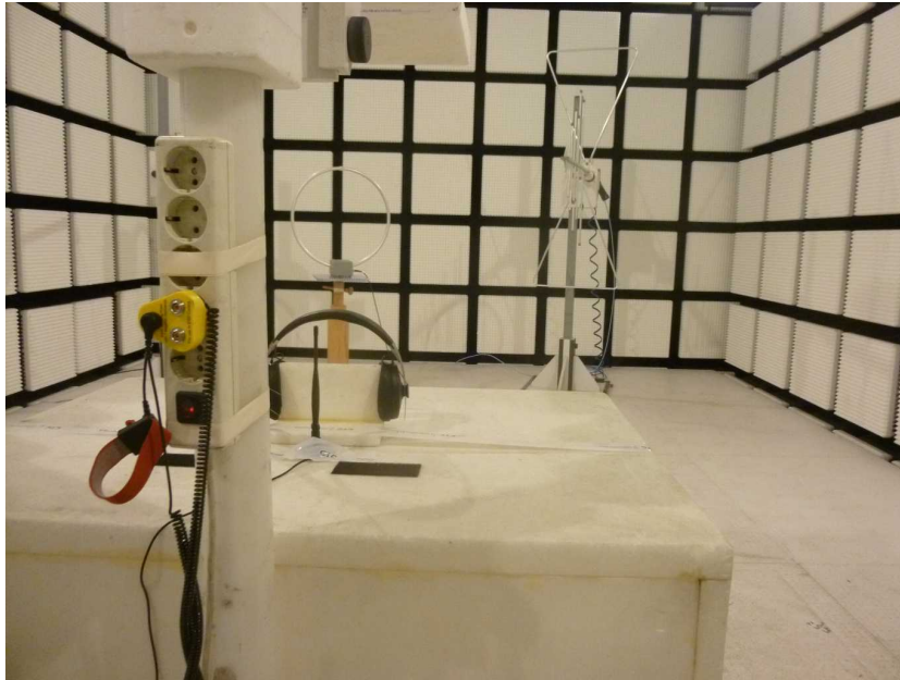
Photo 11: EUT at the anechoic chamber, loop antenna test setup
