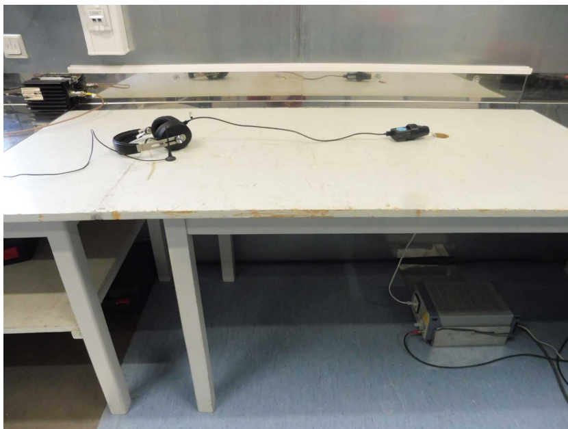
Photo 14: AC conducted emission test setup
