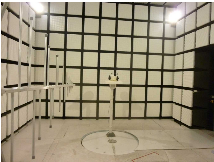
Photo 6: EUT at the anechoic chamber
