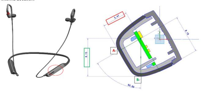
The separation distance for antenna to edge:
