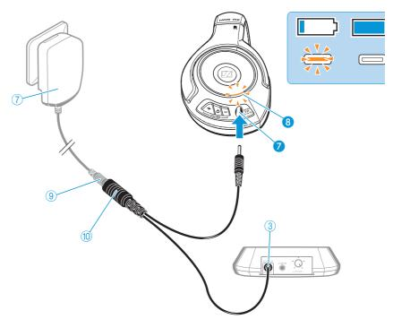
The transmitter automatically switches from battery operation to mains operation if you connect the power supply unit or the charging cable (1) to the transmitter.
