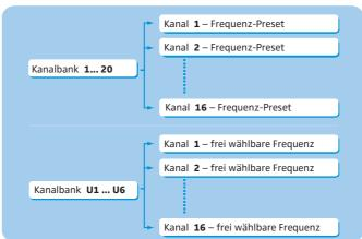
Each of the channels in the frequency banks "1" to "20" has been factory-preset to a fixed transmission frequency (frequency preset). The factory-preset frequencies within one frequency bank are intermodulation-free. These frequencies cannot be changed.
