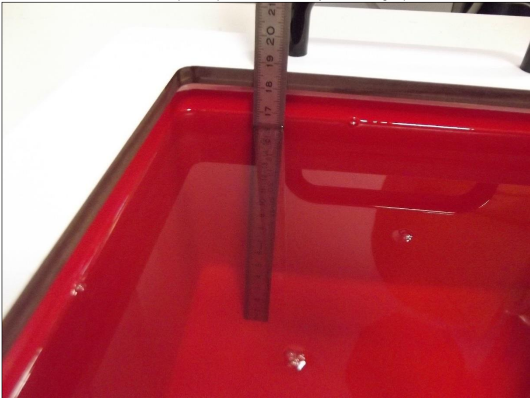
Photo 1: Liquid depth 450 MHz body simulating liquid
