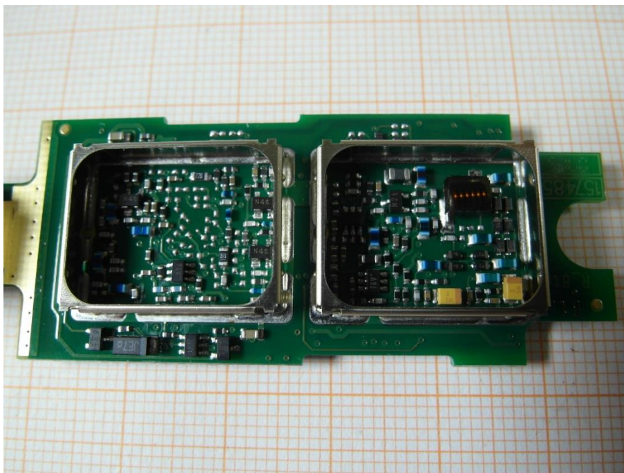
Photo 8: RF part without shielding
