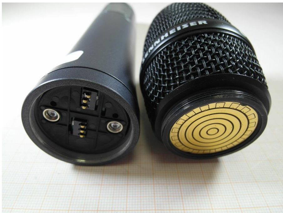
Photo 5: interface microphone to electronic part
