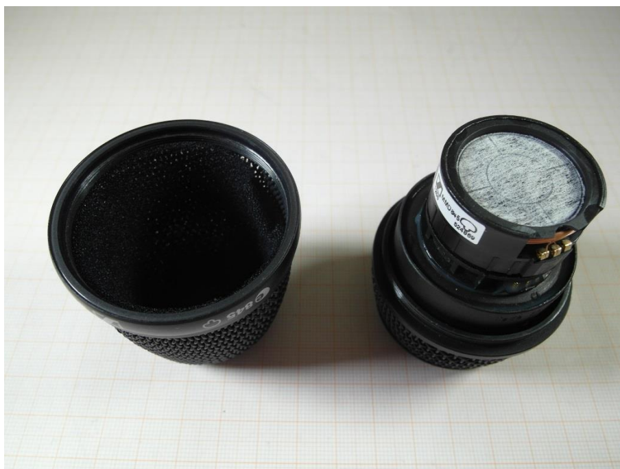
Photo 6: microphone without protection housing
