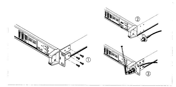
Mounting the transmitter into a rack
