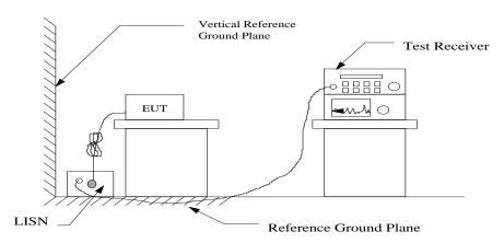
Figure 3 : Conducted emissions measurement configuration
