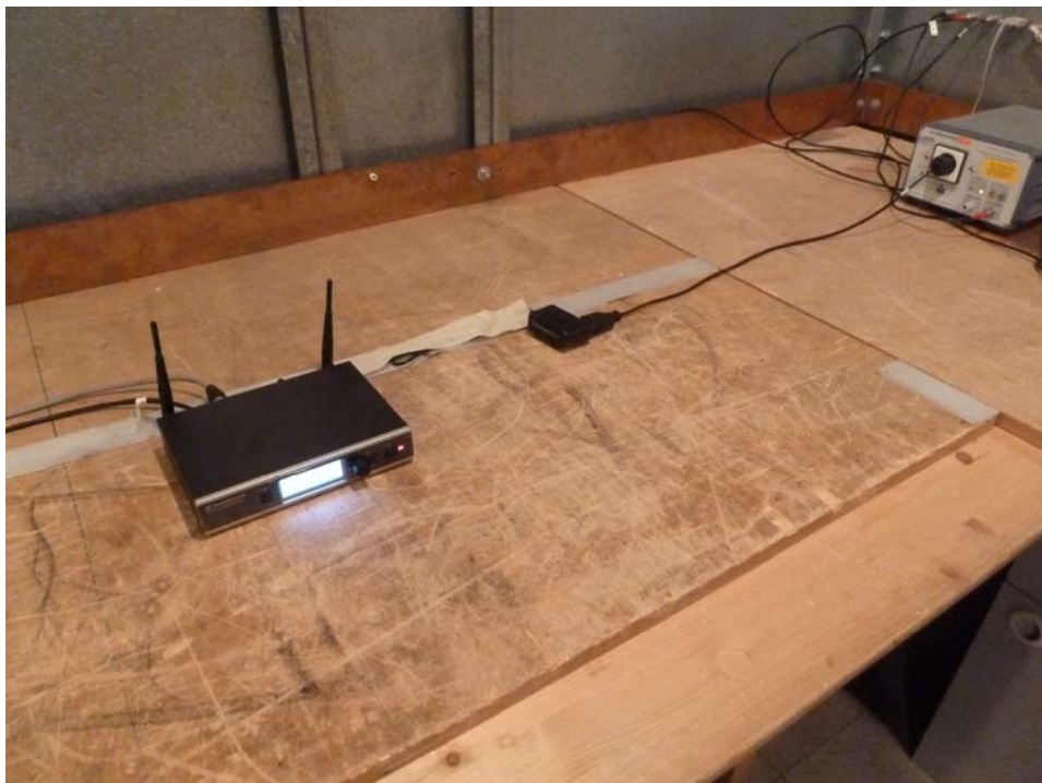
Photo 2: Power Line Conducted Emission Test
