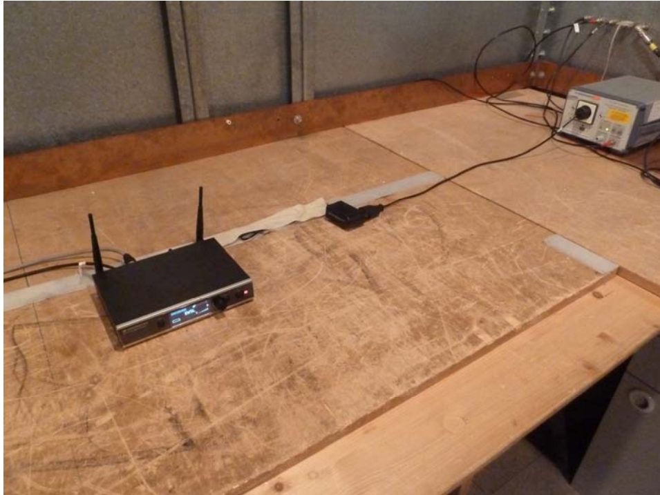
Photo 1: Power Line Conducted Emission Test
