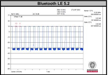
The duty factor of Bluetooth signal has been calculated as following.
