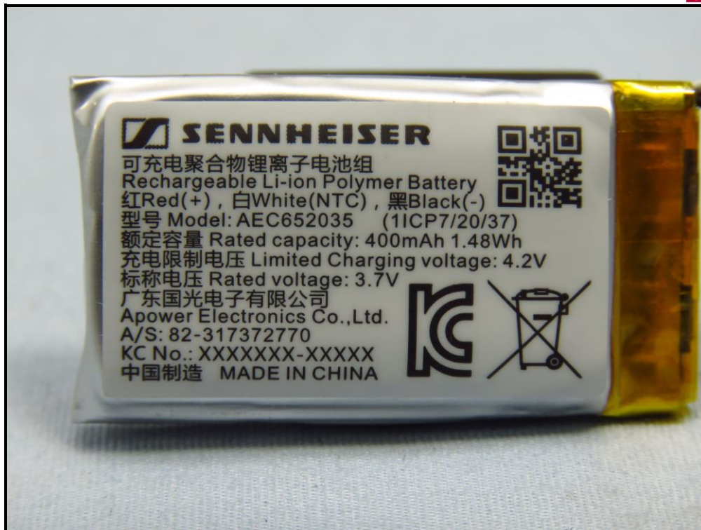
Earbud (alternative battery cell)
