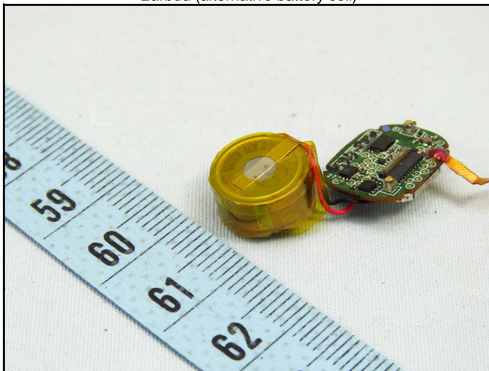
Earbud (alternative battery cell)
