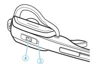
▶ Press the LINK button 4 on the headset. The link is established. The LINK LED 4 lights up blue and the HEADSET LED (3) flashes blue.
