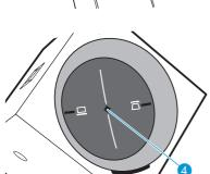
To mute the headset's microphone during a call (the LINK LED 4) on the base station lights up blue):
