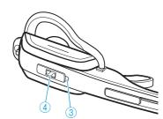
▶ Press and hold the LINK button 4 for 5 seconds. The HEADSET LED 3 flashes blue 3 times and the wireless link to the base station is established (where required). An ascending confirmation beep is heard in the headset.
