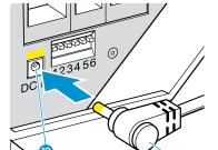
Connect the DC IN connector 6 of the power supply unit to the DC IN socket 2.
