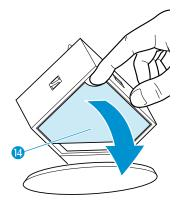
Remove the cover 14 by inserting a finger into the recess as shown.
