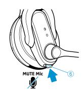
To mute the headset's microphone during a call (the LINK LED 4) on the base station lights up blue):
