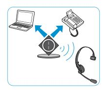
You can use the headset system with your fixed line phone (Phone mode) and/or your PC (PC mode). The base station controls the wireless communication between the products.
