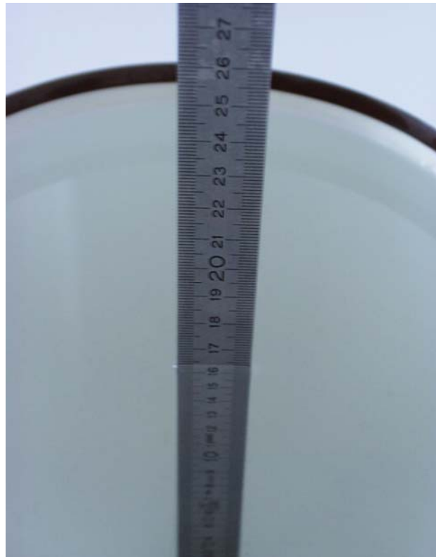
Fig. 15: Liquid depth for 1900 MHz Head measurements.
