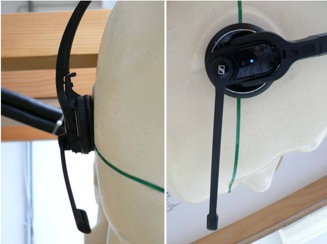
Fig. 14: Cheek position, right side, antenna 1 and 2.
