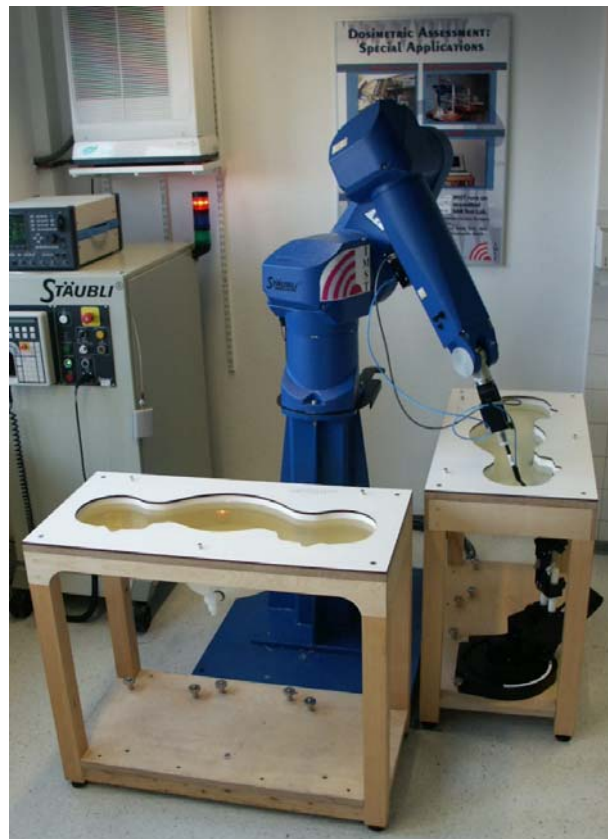
Fig. 7: The measurement set-up with two SAM phantoms containing tissue simulating liquid.
