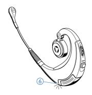
When your mobile device prompts a keyword, enter four zeros (0000). When pairing was successful, the headset LED (6) lights up blue 3 times. The headset acknowledges with a tone, and your mobile device displays a message.
