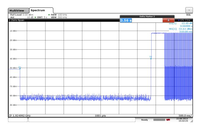
7.3.4 Selected Channel Confirmation, Connection 3.6s After Interferer Removed
