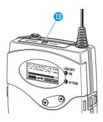
Set the MUTE switch 13 back to the original position to retransmit the audio signal.
