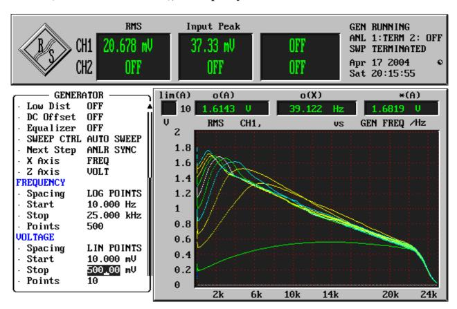
max. measured frequency deviation: 41.6 kHz
