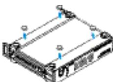
The device feet are fitted to the base of the AC 3 (see diagram).
