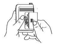
**Step 2.** Using the supplied screwdriver, set the Channel setting switch pointer to the desired channel number.
