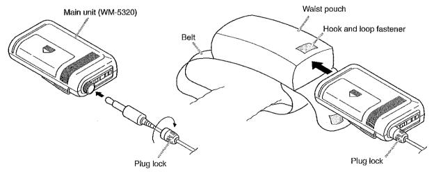
Secure the connection with the plug lock.
