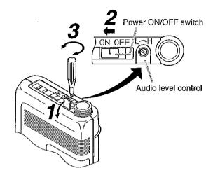
Step 4. Adjust the corresponding tuner's volume control so that its knob points to the 2 o'clock position. If the tuner's AF PEAK indicator remains lit, readjust the microphone's audio level control to the position that causes the indicator to flash when the tuner output level reaches its peak. The AF PEAK indicator lights when the output level reaches the point of about 3 dB below the clipping level.
