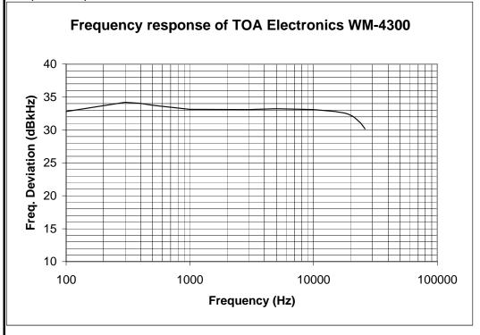
Peak is at 300 Hz. Maximum deviation at this frequency is 51.4 kHz 50% is 25.7 kHz deviation. 16 dB additional drive is added and the modulation applied at 25000 Hz
