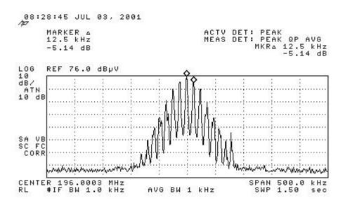
Plots above are for 74.861. Fundamental frequency set at 196 MHz with a 12.5 kHz tone
