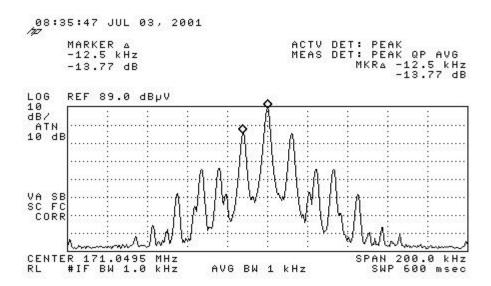
Plots above are for 90.265. Fundamental frequency set at 171 MHz with a 12.5 kHz tone
