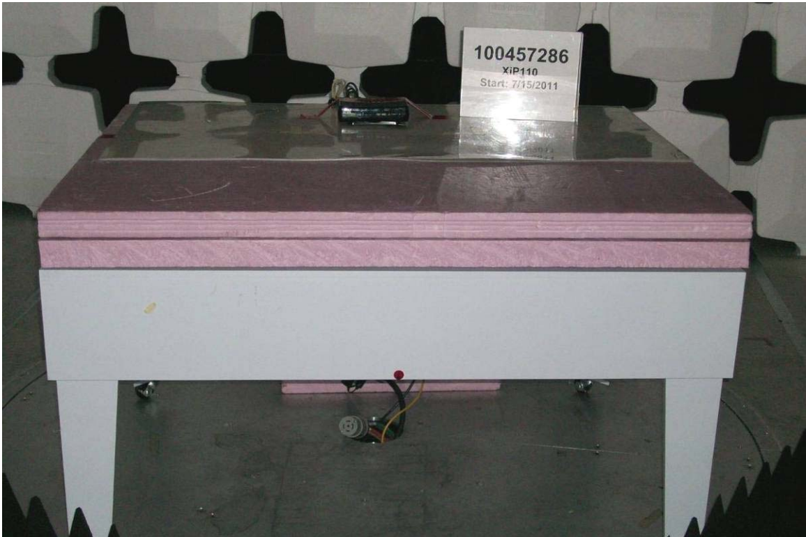
Test Setup – Radiated Emissions (Front View)
