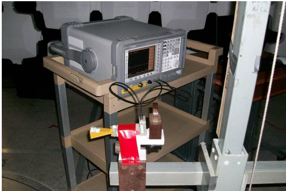
HF Active Antenna/Harmonic Mixer (18GHz – 26.5GHz)
