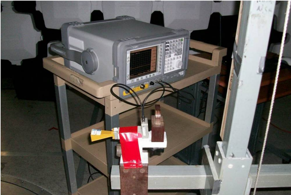
HF Active Antenna/Harmonic Mixer (18GHz – 26.5GHz)
