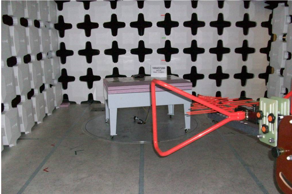
Ridge Guide Horn (1GHz to 18GHz)
