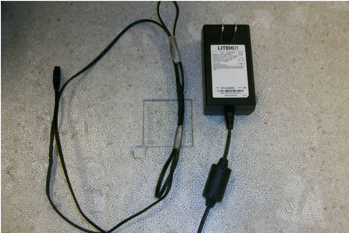
AC Adapter – 12VDC Output
