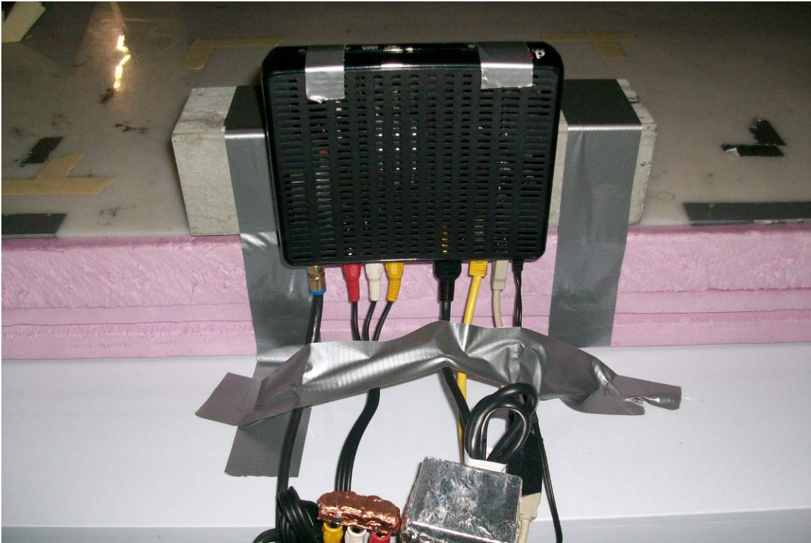
Test setup – Field Strength Measurements (Rear View Cables)
