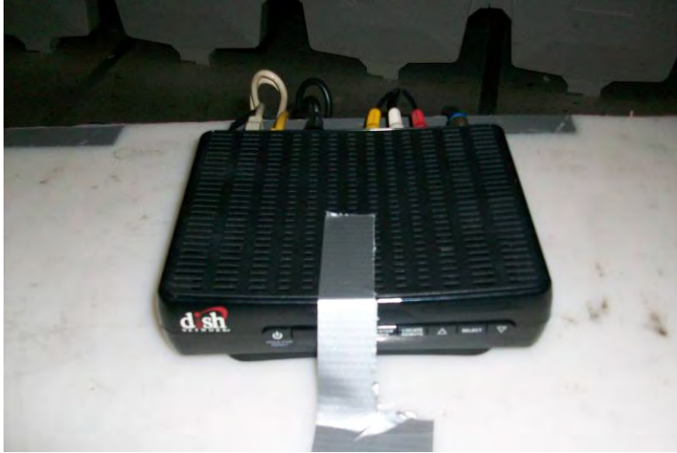
Test Axis 2 (Product Vertical)
