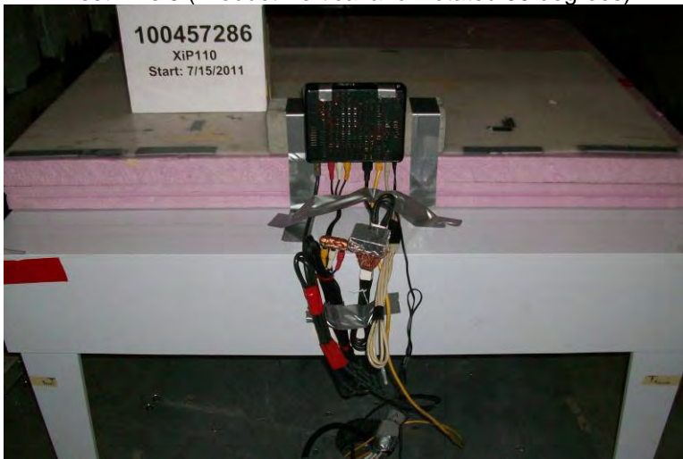
Axis 3 was determined to be the "worst-case" product orientation
