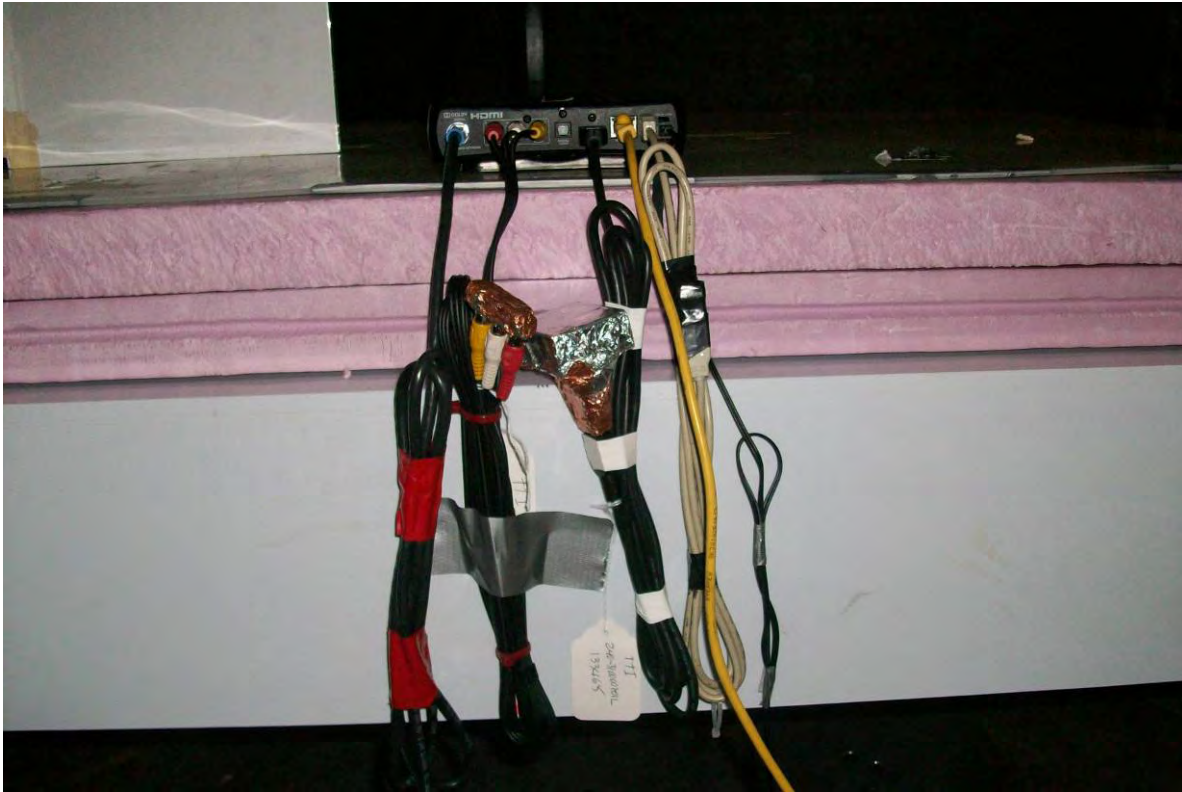
Cables Left-to-Right: RF Coaxial, Composite A/V RCA, HDMI, Ethernet, USB, DC Power
