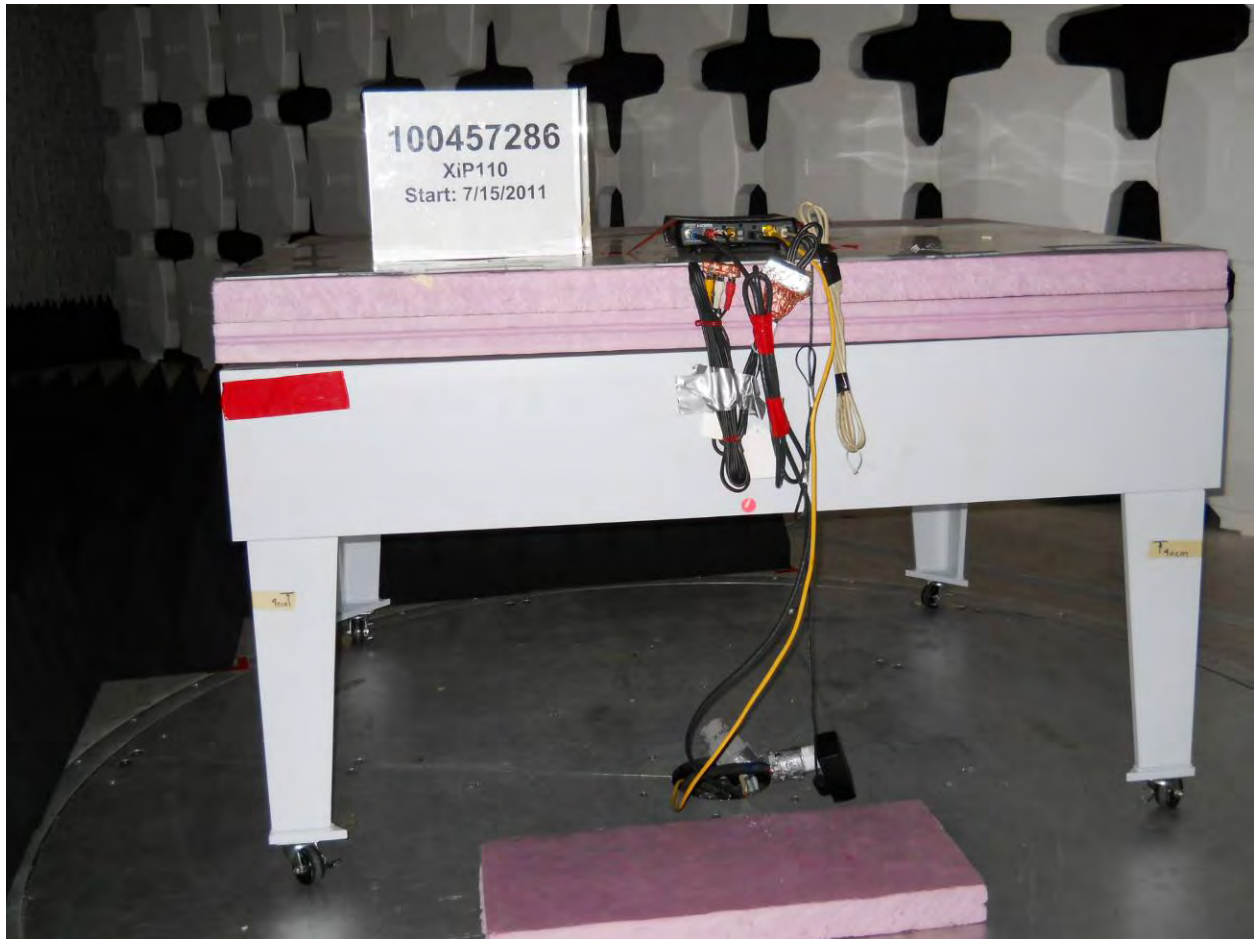
Test Setup – Radiated Emissions (Rear View)
