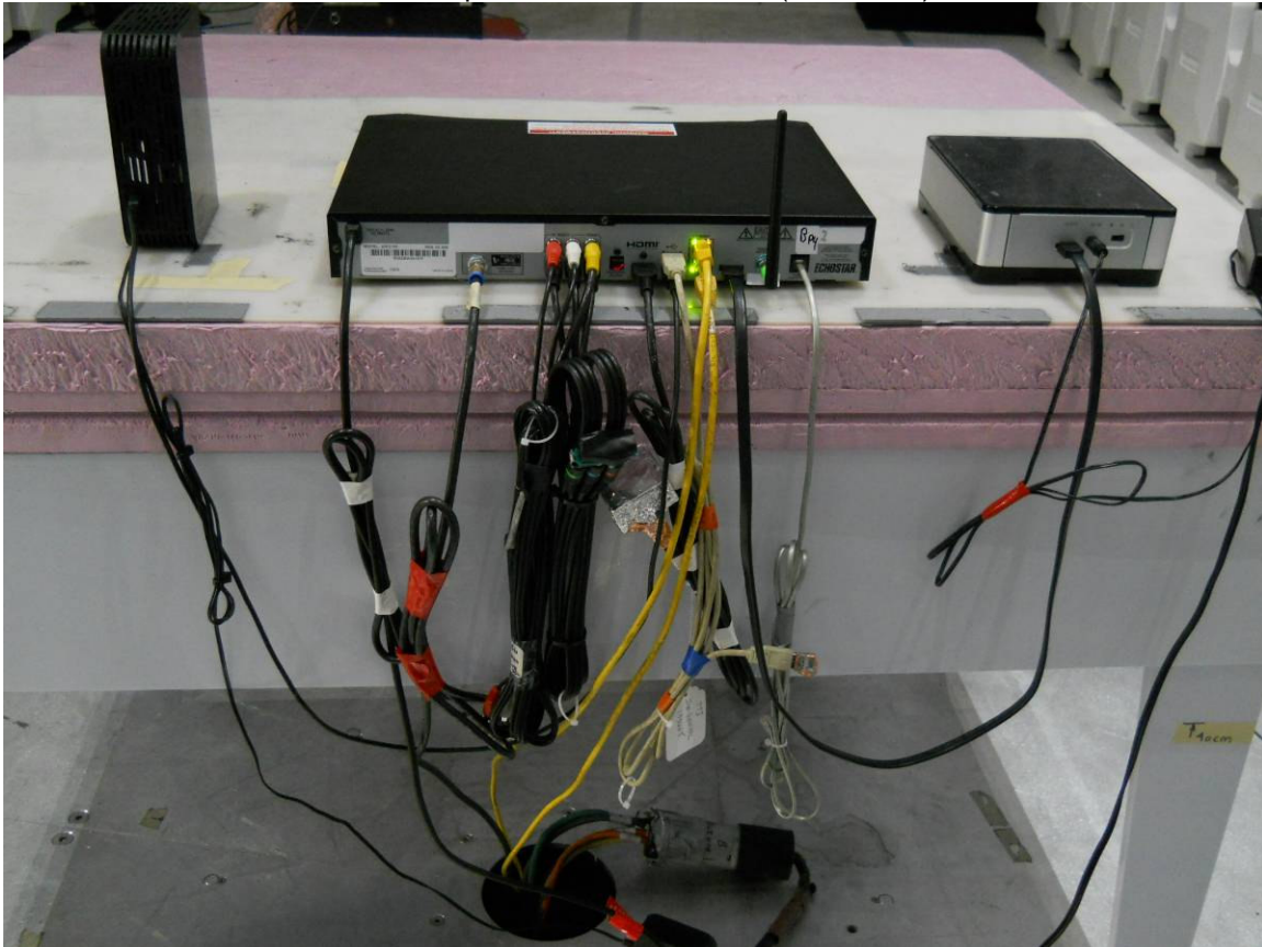
Test Setup – Radiated Emissions (Rear View)
