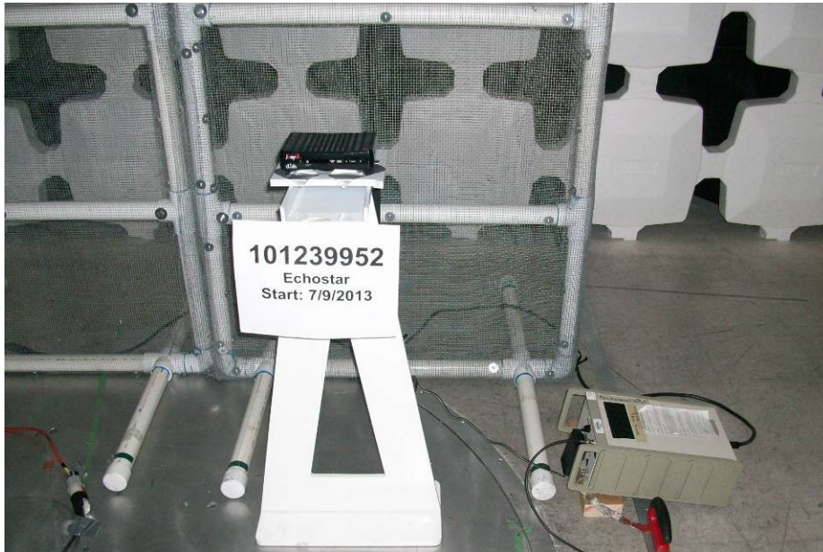
Test Setup – AC Conducted Emissions (Front View)
