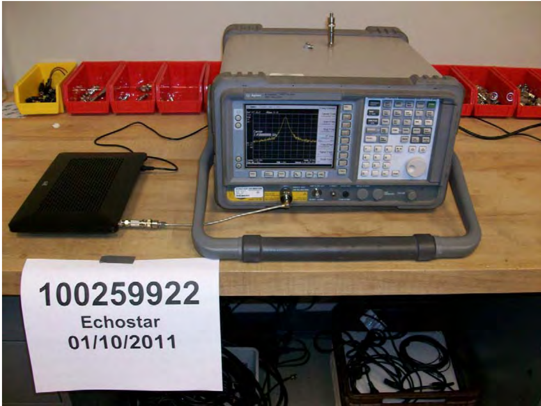
Test setup – RF Conducted Port Measurements
