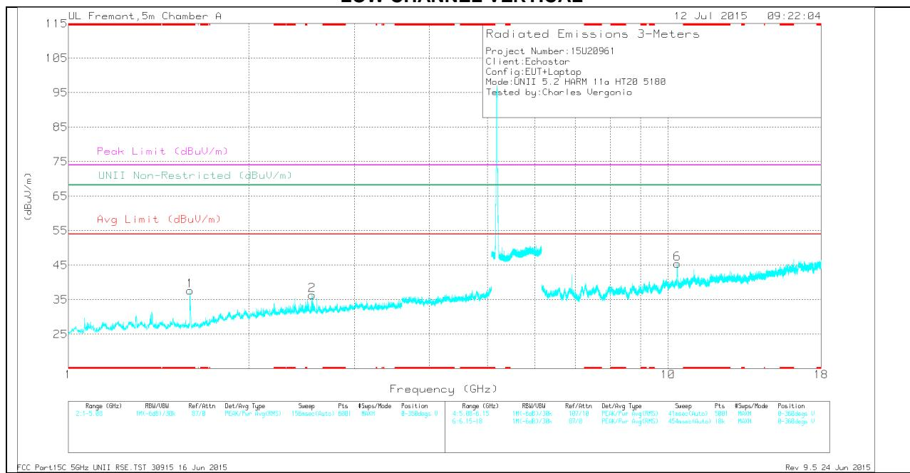
Note: Emission was scanned up to 40GHz; No emissions were detected above the noise floor which was at least 20dB below the specification limit.
