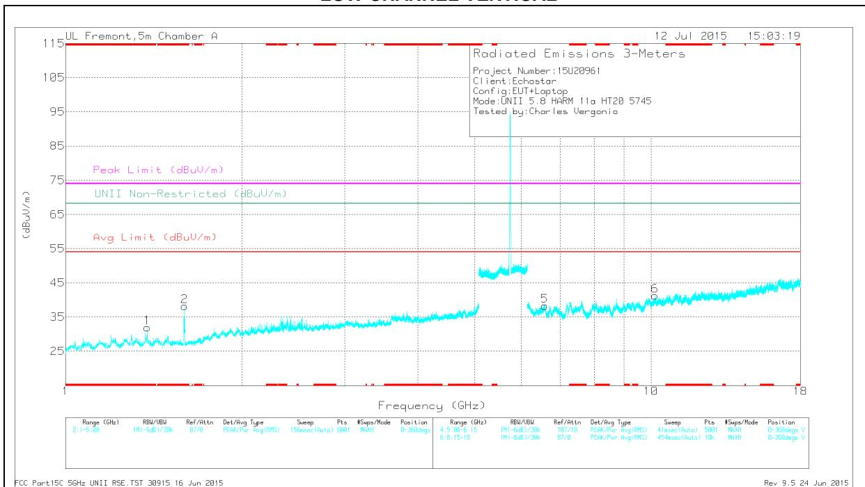
Note: Emission was scanned up to 40GHz; No emissions were detected above the noise floor which was at least 20dB below the specification limit.
