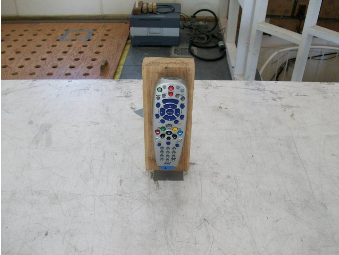
Test Setup – Axis 3: EUT Vertical & Rotated 90 Degrees
