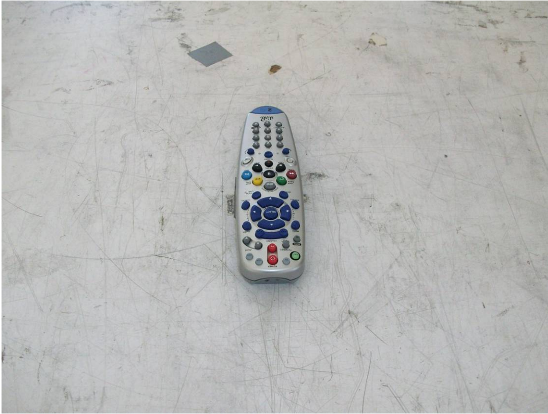
Test Setup – Axis 1: EUT Flat on Table
