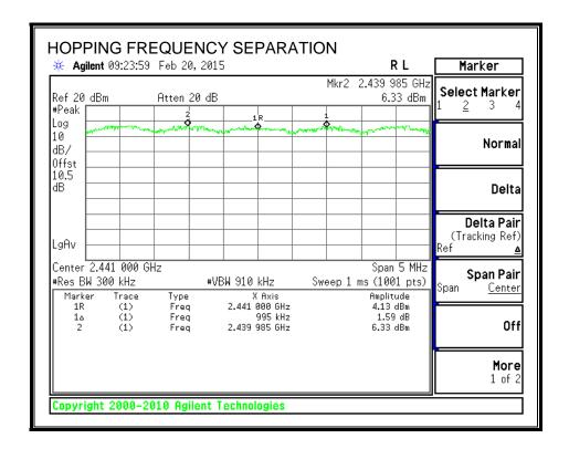
Note – The EUT's Channel separation (995 kHz) is less than the 20 dB bandwidth (1.299 MHz). However, the EUT's power is less than 125 mW or 20 dBm (Power approx. 8 dBm). Therefore, the channel separation is allowed to be greater than 2/3's the 20 dB BW or 866 kHz.
