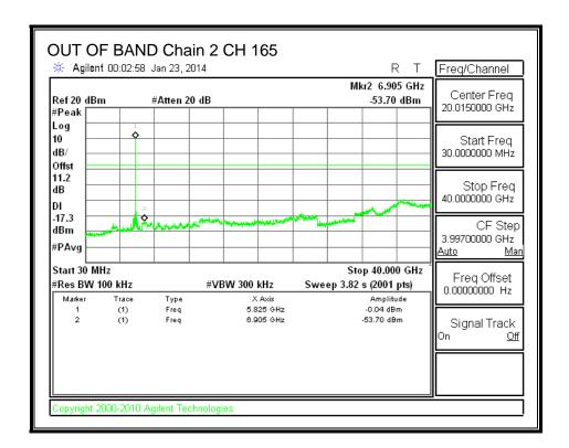
REPORT NO: 13U16571-1 EUT: 802.11ac 3x3 Set Top Box Client with RF4CE for remote operation
